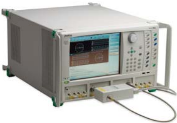
Figure 3. A typical AutoCal setup is shown here.
